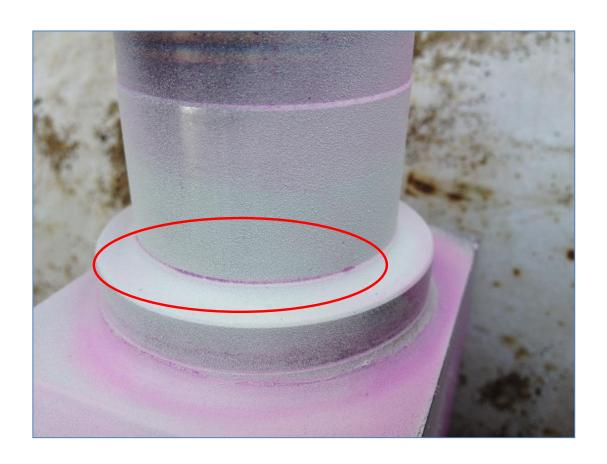
Final confirmation with LPT to detect surface cracks
