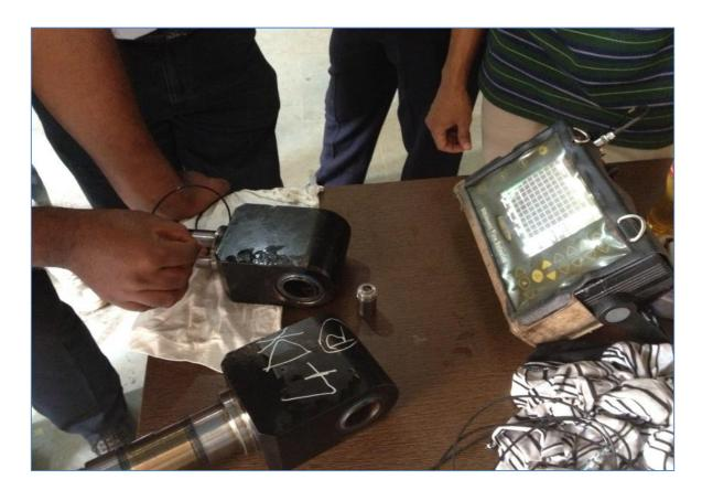
UFD carried out to identify subsurface cracks, voids, porosities
